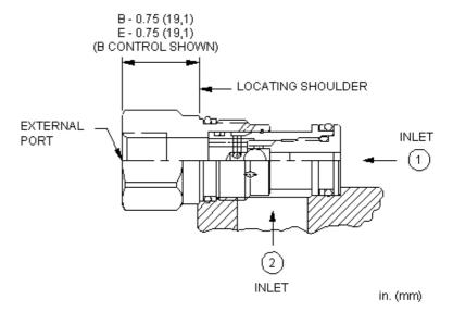
The single ball shuttle connects the higher of two work ports to the signal or common port. The signal is sensed at an external port located in the hex-end of the cartridge.
