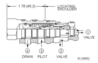
This is a normally closed, balanced poppet, switching element. When the vent port (port 4) is blocked, the poppet remains in the closed position. Venting port 4 shifts it to the open position, provided there is sufficient pressure at port 3.
