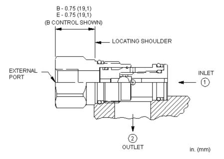
The single ball shuttle connects the higher of two work ports to the signal or common port. It features an external load port located in the hex-end of the cartridge and the signal is sensed at port 2.
