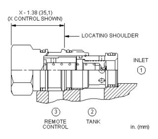
Normally closed modulating elements with an internal orifice between port 1 and port 3 can be used as a mainstage relief valve. The valve can be controlled remotely using a pilot relief or pilot solenoid valve.
