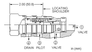
This is a normally open, balanced poppet, switching element. When the vent port (port 4) is blocked, the poppet remains in the open position. Venting port 4 shifts it to the closed position, provided there is sufficient pressure at port 3.
