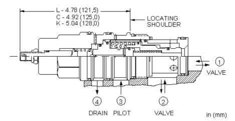
This is a normally closed, balanced poppet, switching element. When pilot pressure is applied to port 3, the poppet remains closed until the pilot pressure reaches the setting established by the integral pilot relief stage, at which point the poppet shifts to the open position.
