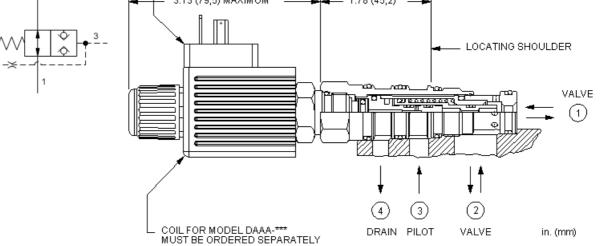
This is a normally open, balanced poppet, switching element with an integral T-8A control cavity. With a 2-way valve in the closed position installed in the T-8A control cavity, the poppet remains open. Opening the 2-way valve shifts the poppet to the closed position, provided there is sufficient pressure at port 3.
