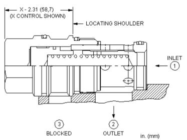
Free-flow, nose-to-side cheater check valves function as a standard 2-port check valve in a 3-port cavity with port 3 of the cartridge blocked off. These valves are useful in circuits where a check valve is required in an existing three port cavity.
