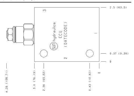
Counterbalance valves with pilot assist are meant to control an overrunning load. The check valve allows free flow from the directional valve (port 2) to the load (port 1) while a direct-acting, pilot-assisted relief valve controls flow from port 1 to port 2. Pilot assist at port 3 lowers the effective setting of the relief valve at a rate determined by the pilot ratio.
