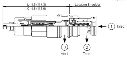
Ventable, pilot-operated, anti shock relief cartridges limit maximum system pressure and also limit the rate of pressure rise. The valve opens and then ramps closed at a constant speed, independent of settings and flows. These 3 port valves include a vent port (port 3) that connects between the main piston and the pilot stage to provide for remote control by other pilot or 2-way valves. The adjust screw determines the maximum (relief) setting and the minimum (threshold) setting.
