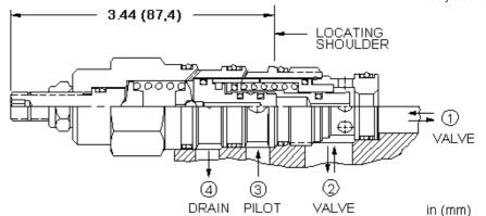
This is a normally open, balanced poppet, switching element. When pilot pressure is applied to port 3, the poppet remains open until the pilot pressure reaches the setting established by the integral pilot relief stage, at which point the poppet shifts to the closed position.
