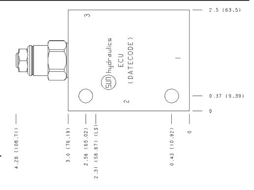
Counterbalance valves with pilot assist are meant to control an overrunning load. The check valve allows free flow from the directional valve (port 2) to the load (port 1) while a direct-acting, pilot-assisted relief valve controls flow from port 1 to port 2. Pilot assist at port 3 lowers the effective setting of the relief valve at a rate determined by the pilot ratio.
