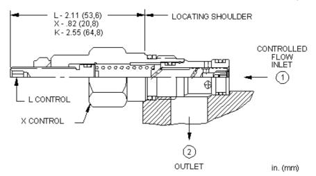
Fixed-orifice, pressure-compensated flow controls provide precise flow regulation for meter-in or meter-out applications where there may be wide pressure fluctuations. The flow setting is specified by the user and is set at the factory.
