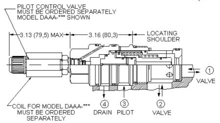
This is a normally open, balanced poppet, switching element with an integral T-8A control cavity. With a 2-way valve in the closed position installed in the T-8A control cavity, the poppet remains open. Opening the 2-way valve shifts the poppet to the closed position, provided there is sufficient pressure at port 3.
