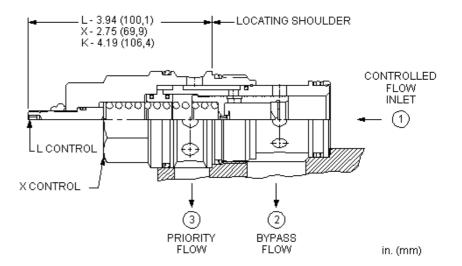
Bypass/restrictive, fixed-orifice, priority flow controls take an input flow at port 1 and use it to satisfy the priority flow at port 3. If the input flow exceeds the priority flow requirement, the excess is bypassed out port 2. The bypass flow may be used in a secondary circuit.
