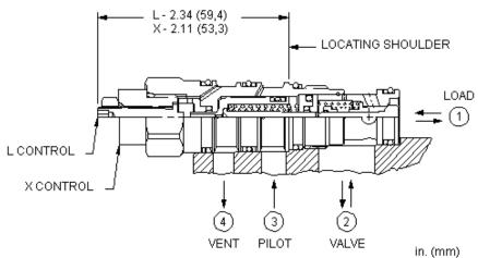
This valve is a pilot to open check valve. It has a sealed pilot, a steel seat, and is vented. It allows free flow from the valve (port 2) to the load (port 1) and blocks flow in the opposite direction. Pressure at the pilot (port 3) will open the valve from port 1 to port 2. Pilot pressure needed to open the valve is directly proportional to the load pressure at port 1. The valve is insensitive to pressure at port 2 because the spring chamber is referenced to the vent (port 4).
