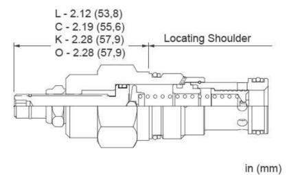
Pilot-operated, balanced-piston relief cartridges are normally closed pressure regulating valves. When the pressure at the inlet (port 1) reaches the valve setting, the valve starts to open to tank (port 2), throttling flow to regulate the pressure. These valves are accurate, have low pressure rise vs. flow, they are smooth and quiet, and are moderately fast.
