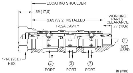
High-capacity, closed-center flow divider/combiners are sliding-spool, pressure-compensated devices used to split flow in one direction and combine flow in the opposite direction. These valves have approximate 15% greater capacity than standard closed-center divider/combiners and are designed for use in tractive drive systems. Note: Accuracy on these cartridges is not equivalent to the accuracy of standard closed-center divider/combiners.
