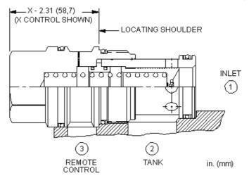
Normally closed modulating elements with an internal orifice between port 1 and port 3 can be used as a mainstage relief valve. The valve can be controlled remotely using a pilot relief or pilot solenoid valve.
