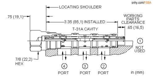
Closed-center flow divider/combiners are sliding-spool, pressure-compensated devices used to split flow in one direction and combine flow in the opposite direction. These valves may be used to accurately control two or more cylinders or hydraulic motors where bidirectional operation is required.
