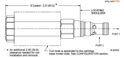
This valve is a pilot-operated, normally closed, electro-proportional throttle with reverse free-flow check. Energizing the coil generates an opening force on the pilot stage which vents the main stage poppet to open proportionally, allowing flow from port 2 to 1. The check will allow flow from 1 to 2 in either the open or closed condition.
