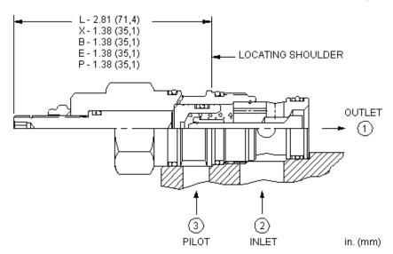
This valve is a pilot to open check valve. It has a sealed pilot, a steel seat, and is non-vented. It allows free flow from the valve (port 2) to the load (port 1) and blocks flow in the opposite direction. Pressure at the pilot (port 3) will open the valve from port 1 to port 2. Pilot pressure needed at port 3 to open the valve is directly proportional to the load pressure at port 1. Pressure at port 2 directly opposes pilot pressure.
