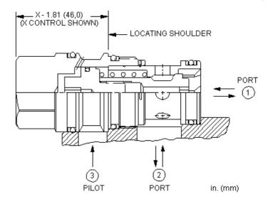
These unbalanced poppet, logic valves are 2-way switching elements that are spring-biased closed. Pressure at either work port 1 or 2 will further bias the valve to the closed position while pressure at port 3 will tend to open it. The force generated at port 3 must be greater than the sum of the forces acting at port 1 and port 2 plus the spring force for the valve to open. NOTE: The pilot area (port 3) is 1.8 times the area at port 1 and 2.25 times the area at port 2.
