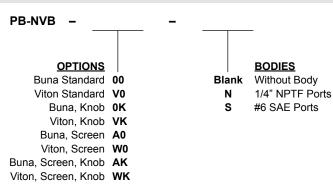
Note: use screen only if flow direction is from (1) to (2).
