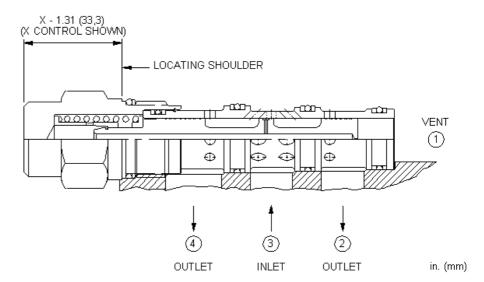
This vent-to-shift diverter valve is a 2-position, 3-way cartridge that is normally open from port 3 to port 4. When port 1 is vented, the pressure differential between port 3 and port 1 exceeds the spring force causing the valve to shift, thereby connecting port 3 to port 2.
