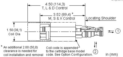
This solenoid-operated 2-way, 2-position cartridge is a direct-acting, balanced spool directional valve. The valve is available in either a normally open or normally closed configuration.
