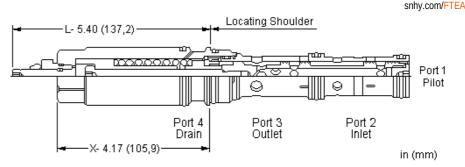
This valve is a 2-way, 2-position proportional throttle. Pilot pressure at port 1 opposes the spring and creates a variable metering orifice between port 2 and 3 that is proportional to the pressure at 1. The force balance of the flow forces, spring and pilot pressure results in a degree of partial self-compensation as the load pressure changes.
