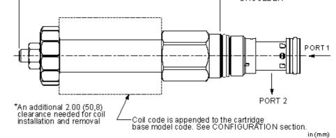
This FLeX Series solenoid-operated, 2-stage, balanced relief cartridge is a pressure regulating valve.
