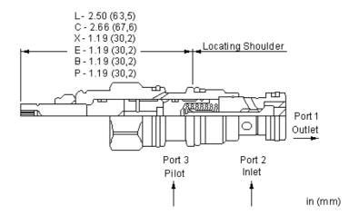
This valve is a pilot to open check valve. It has a sealed pilot, a steel seat, and is non-vented. It allows free flow from the valve (port 2) to the load (port 1) and blocks flow in the opposite direction. Pressure at the pilot (port 3) will open the valve from port 1 to port 2. Pilot pressure needed at port 3 to open the valve is directly proportional to the load pressure at port 1. Pressure at port 2 directly opposes pilot pressure.
