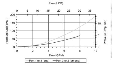
Common lift/lower valve where load holding is not required. For higher pressures see HF-S3A.
