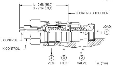
This valve is a pilot to open check valve. It has a sealed pilot, a steel seat, and is vented. It allows free flow from the valve (port 2) to the load (port 1) and blocks flow in the opposite direction. Pressure at the pilot (port 3) will open the valve from port 1 to port 2. Pilot pressure needed to open the valve is directly proportional to the load pressure at port 1. The valve is insensitive to pressure at port 2 because the spring chamber is referenced to the vent (port 4).
