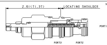
Normally open modulating elements without an internal orifice act as a restrictive compensator to maintain a constant pressure drop across an orifice, regardless of variations in upstream or downstream pressure.
