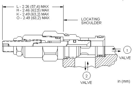
Needle valves are fully adjustable orifices used to regulate flow. They are infinitely adjustable from fully closed up to the maximum orifice diameter. They are not pressure compensated and may be used as flow controls or as shutoff valves.
