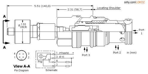
These unbalanced, pilot-to-close logic valves are 2-way switching elements that are spring biased open. Pressure at either work port 1 or 2 will tend to keep the valve open while pressure at port 3 will tend to close it. The force generated at port 3 must be greater than the sum of the forces acting at port 1 and port 2 plus the spring force for the valve to close. NOTE: The pilot area (port 3) is 1.8 times the area at port 1 and 2.25 times the area at port 2.
