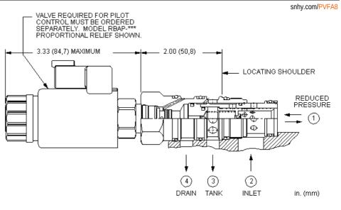
This valve is a 3-way, normally open modulating element, externally drained, that incorporates an integral pilot control cavity. The pilot control cavity will accept any T-8A pressure control cartridge. The valve reduces a high primary pressure at the inlet (port 2) to a constant reduced pressure at port 1, with a full flow relief function from port 1 to tank (port 3). The pilot cartridge's setting determines the difference in pressure between reduced pressure (port 1) and the drain (port 4).
