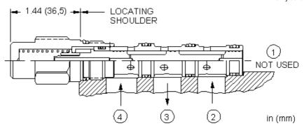
Spring-offset, high-side shuttle cartridges are 2-position valves that have a normal (offset) position that connects the common port (port 3) to work port 4, with work port 2 blocked. When the pressure at port 2 rises above the pressure at port 4, the cartridge shifts to connect the common port to port 2 with port 4 then blocked.
