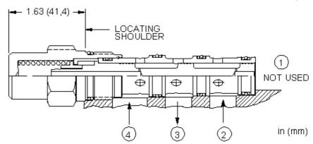
Spring-offset, high-side shuttle cartridges are 2-position valves that have a normal (offset) position that connects the common port (port 3) to work port 4, with work port 2 blocked. When the pressure at port 2 rises above the pressure at port 4, the cartridge shifts to connect the common port to port 2 with port 4 then blocked.
