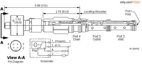
This valve is a 2-way, 2-position proportional throttle. Ports 2 and 3 are normally closed. Pilot pressure at port 1 creates a metering orifice between port 2 and 3 that is proportional to the pressure at 1. The metering passage is self-compensating.
