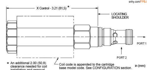
This valve is a pilot-operated, normally open, electro-proportional throttle with reverse free-flow check. Energizing the coil generates a closing force on the pilot stage which pushes the main stage poppet against the seat, proportionally blocking flow from port 2 to 1. The check will allow flow from 1 to 2 in either the open or closed condition.
