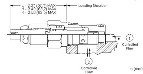
Needle valves are fully adjustable orifices used to regulate flow. They are infinitely adjustable from fully closed up to the maximum orifice diameter. They are not pressure compensated and may be used as flow controls or as shutoff valves.
