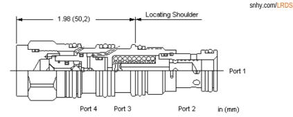
A normally closed modulating element, used as a bypass compensator, ensures a constant pressure drop across an external orifice to create a pressure compensated flow control. The resulting flow remains constant regardless of variations in upstream or downstream pressure.
