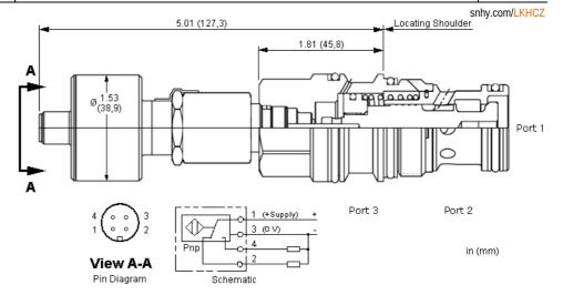
These unbalanced poppet, logic valves are 2-way switching elements that are spring-biased closed. Pressure at either work port 1 or 2 will further bias the valve to the closed position while pressure at port 3 will tend to open it. The force generated at port 3 must be greater than the sum of the forces acting at port 1 and port 2 plus the spring force for the valve to open. NOTE: The pilot area (port 3) is 1.8 times the area at port 1 and 2.25 times the area at port 2.
