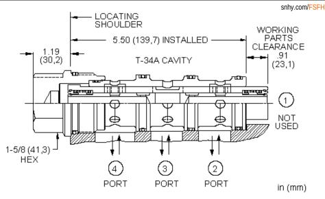
High-capacity, closed-center flow divider/combiners are sliding-spool, pressure-compensated devices used to split flow in one direction and combine flow in the opposite direction. These valves have approximate 15% greater capacity than standard closed-center divider/combiners and are designed for use in tractive drive systems. Note: Accuracy on these cartridges is not equivalent to the accuracy of standard closed-center divider/combiners.
