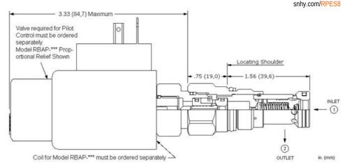
This valve is a normally closed modulating element that incorporates an integral pilot control cavity. It is a balanced poppet design. The pilot control cavity will accept any T-8A pressure control cartridge. When the pressure at the inlet (port 1) reaches the pilot control cartridge's setting, the poppet element starts to open to tank (port 2), throttling flow to regulate the pressure. The pilot cartridge's setting determines the difference in pressure between port 1 and
