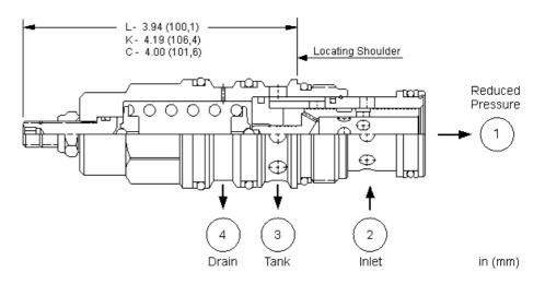
Direct-acting, pressure reducing/relieving valves reduce a high primary pressure at the inlet (port 2) to a constant reduced pressure at port 1, with a full-flow relief function from port 1 to tank (port 3). Draining port 4 makes the valve insensitive to pressure at port 3. These valves incorporate a damped construction for stable operation allowing the use of high reduced pressure.
