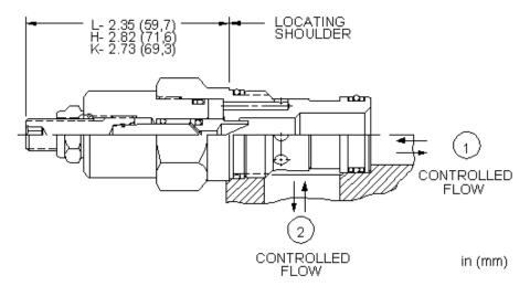
Needle valves are fully adjustable orifices used to regulate flow. They are infinitely adjustable from fully closed up to the maximum orifice diameter. They are not pressure compensated and may be used as flow controls or as shutoff valves.
