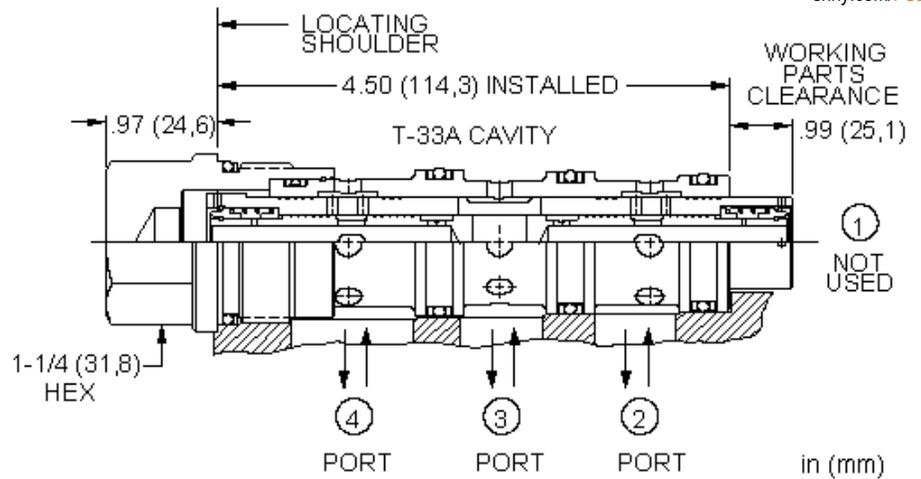
High-capacity, closed-center flow divider/combiners are sliding-spool, pressure-compensated devices used to split flow in one direction and combine flow in the opposite direction. These valves have approximate 15% greater capacity than standard closed-center divider/combiners and are designed for use in tractive drive systems. Note: Accuracy on these cartridges is not equivalent to the accuracy of standard closed-center divider/combiners.
