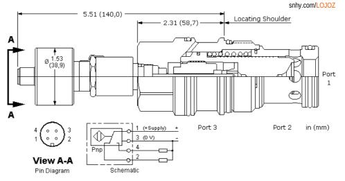
These unbalanced, pilot-to-close logic valves are 2-way switching elements that are spring biased open. Pressure at either work port 1 or 2 will tend to keep the valve open while pressure at port 3 will tend to close it. The force generated at port 3 must be greater than the sum of the forces acting at port 1 and port 2 plus the spring force for the valve to close. NOTE: The pilot area (port 3) is 1.8 times the area at port 1 and 2.25 times the area at port 2.
