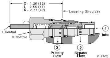
Bypass/restrictive, fixed-orifice, priority flow controls take an input flow at port 1 and use it to satisfy the priority flow at port 3. If the input flow exceeds the priority flow requirement, the excess is bypassed out port 2. The bypass flow may be used in a secondary circuit.
