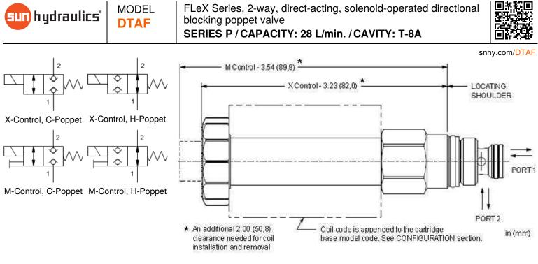
This FLeX Series solenoid-operated 2-way, 2-position cartridge is a direct-acting directional poppet valve. Available in either normally open or normally closed configurations, these valves feature a pressure-balanced design, low leakage, and allow flow or blocking in both directions.
